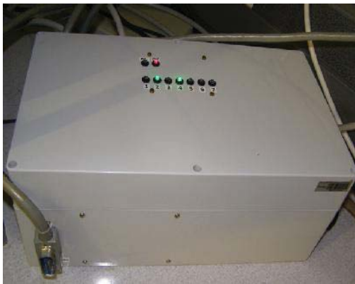
Fig. 4 Programmable GPIB switching isolator (up to 7 channels)
