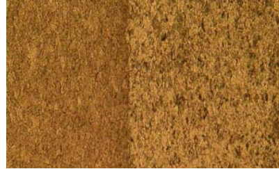
Fig. 4 Interface of specimen welded at 2000RPM
