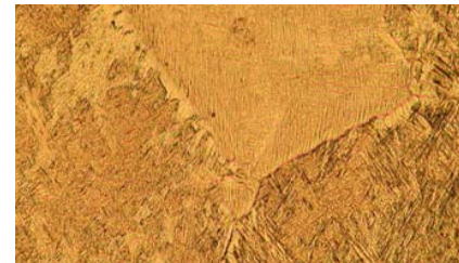
Fig. 6 TZ in the specimen welded at 2000RPM
