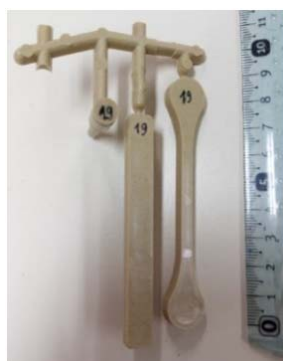
Fig. 1 Injected rod shaped and tensile test WPC samples
