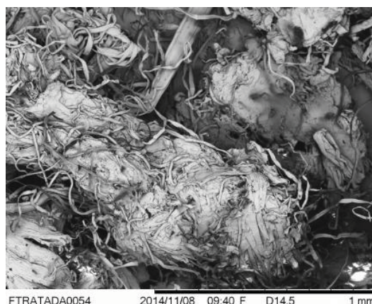
Fig. 2 SEM of the treated fibers 100X
