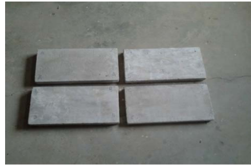
Fig. 3 Sisal fibre-reinforced 4 Concrete slabs
