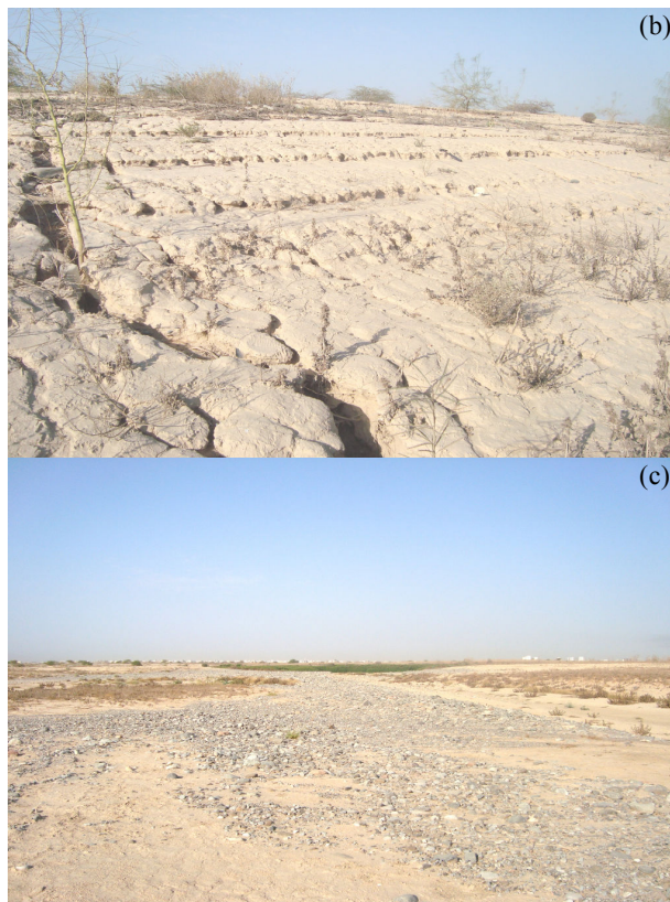
Fig. 6 Field photographs show the occurrences of siltations as (a) clays and (b) layers with (c) the sand and gravels in the Alkhod dam
