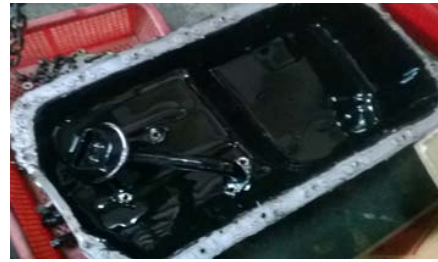
Fig. 6 Contaminates and sludge accumulated in the oil pump
