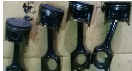
Fig. 8 Dissembled pistons and connecting rods
