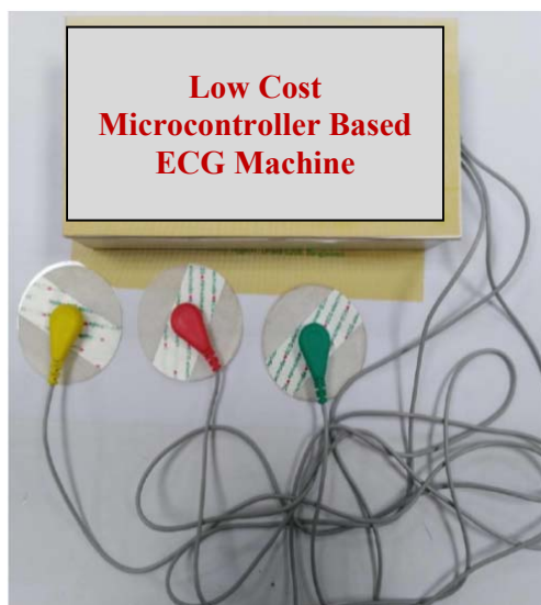
Fig. 5 Complete set-up of the designed ECG machine
