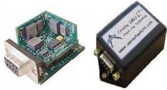
Fig. 6 Cloud Cup Technology Crista IMU which is a very small, low-cost, 3-axis MEMS Inertial Measurement Unit
