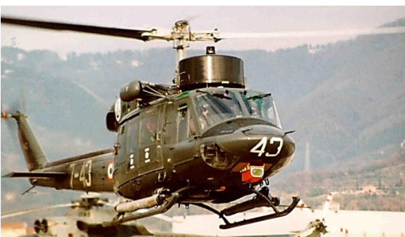
Fig. 18 LOAM installed on AB-212
