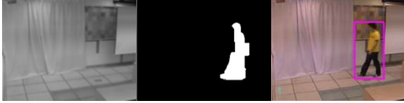
(a) Background (b) Silhouette extraction (c) Object detection Fig. 1 Example of the object detection
