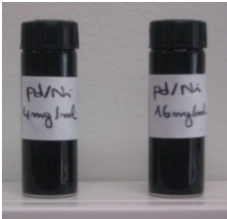
Fig. 1 Photograph of NiPd-Heptane Nanofluids
