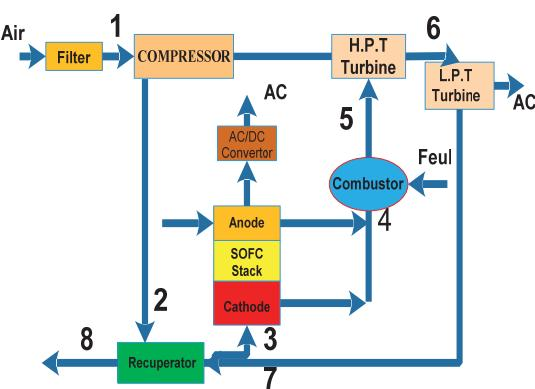
Fig. 1 Detailed schematic diagram of hybrid system
