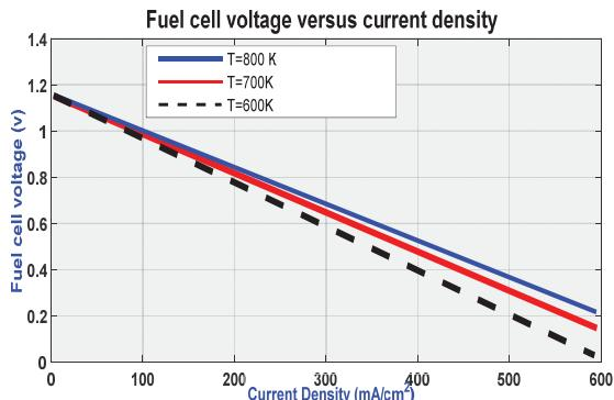
Fig. 2 Voltage of fuel cell according to the current density
