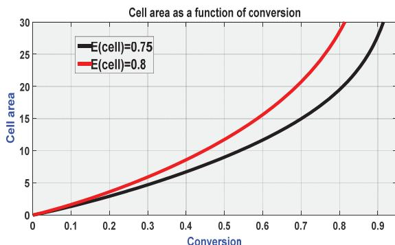
Fig. 8 Functionality of area of fuel cell to converted hydrogen
