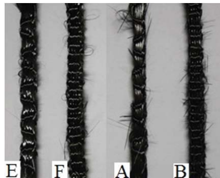
Fig. 5 Non-crimp 3D orthogonal weave samples
