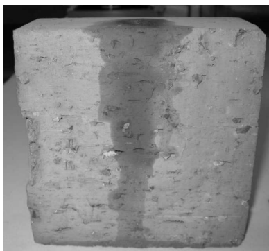
Fig. 1 Ceramic brick filled by siloxane injection
