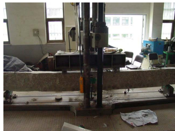
Fig. 5 Four-point loading test of rehabilitated beam
