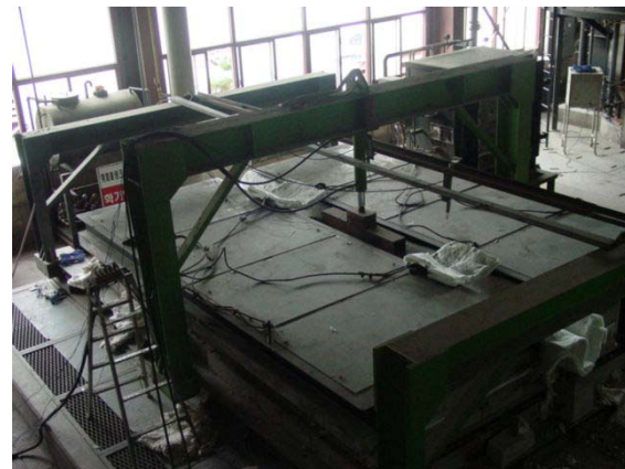
Fig. 4 The horizontal heating furnace for fire test
