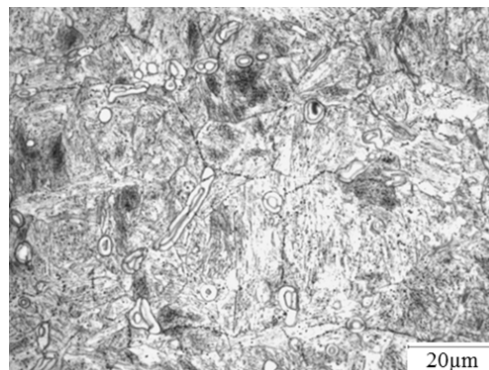
Fig. 7 Detail of microstructure of the sample 1 (1060 °C/30 s without tempering)
