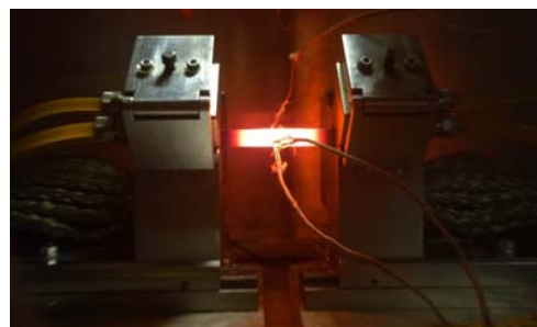
Fig. 2 Sample with thermocouples during heating
