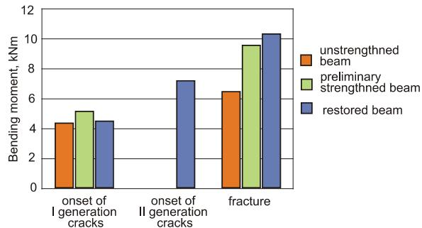
Fig. 9 Critical values of the bending moment
