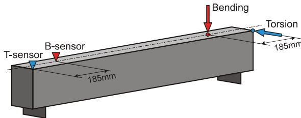
Fig. 3 Scheme of local application of pulse load and the location of the accelerometer
