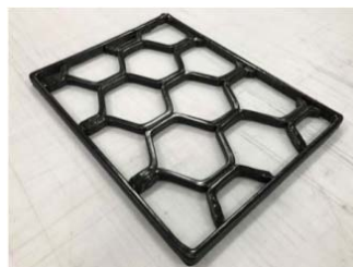
Fig. 1 Prototype 3D printed recycled carbon fiber part
