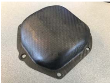
Fig. 7 Completed carbon fiber valve cover
