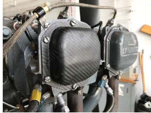
Fig. 14 Test fitting of carbon fiber valve cover
