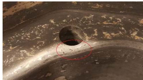
Fig. 10 Mold surface chipping
