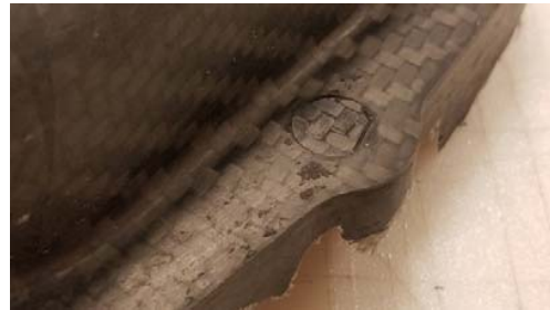
Fig. 8 Surface defects caused by mold surface chipping
