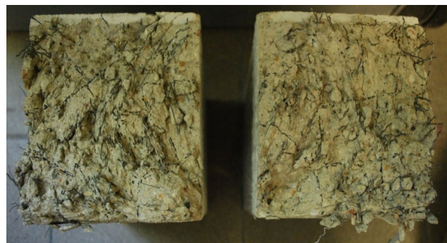
Fig. 8 Both fracture surfaces for one prism. It is possible to see many fibers oriented close to parallel to crack surface. SFRHPC with Tabix50, Dramix30, Dramix13 and Dramix6 fibers (fibers cocktail)
