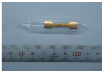
Fig. 3 Appearance of sample for annealing after DSR bonding sealed in quartz tube filled with Ar gas
