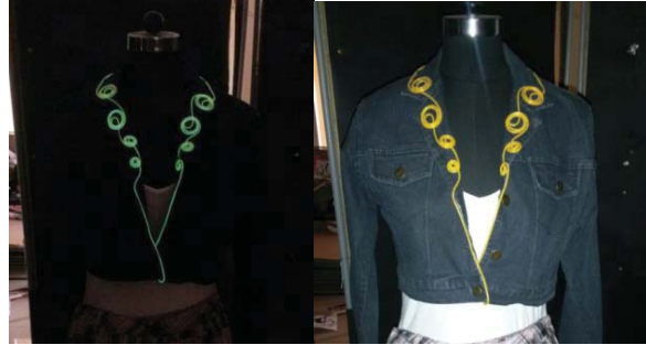
Fig. 9 Denim jacket embedded with EL wire in synchronization to music, thus allowing multiple lengths of EL wire to be flashed in a desired sequence
