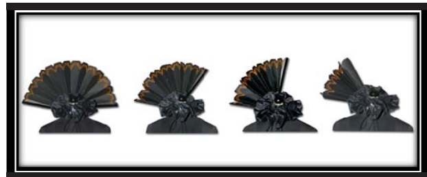
Fig. 6 Movement of the fan with the help of servo motor attached to the neckline which reacts to the proximity sensor
