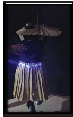
Fig. 5 Pleated skirt Interactive garment integrated with proximity sensors, servomotor and LED's
