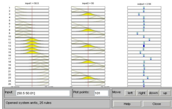
Fig. 10 ANFIS Rule base of Water bath system
