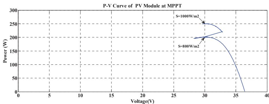
Fig. 9 P-V Characteristics of PV Module at MPPT
