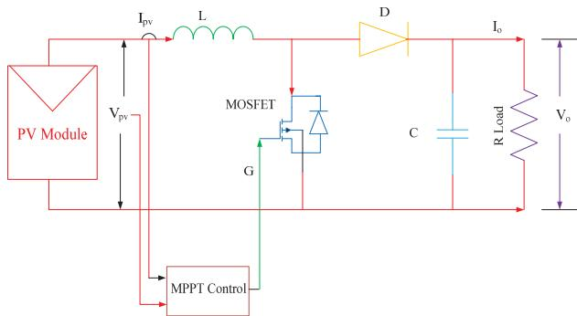
Fig. 4 DC-DC Boost Converter Topology for Proposed MPPT
