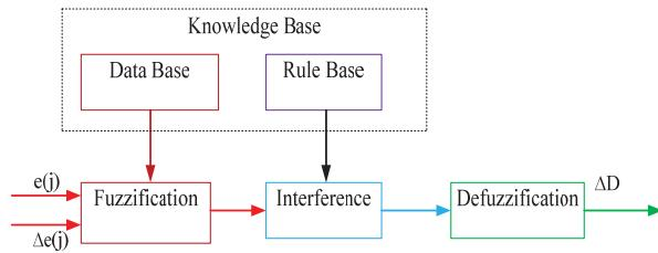
Fig. 5 Block diagram of Fuzzy Inference Systems
