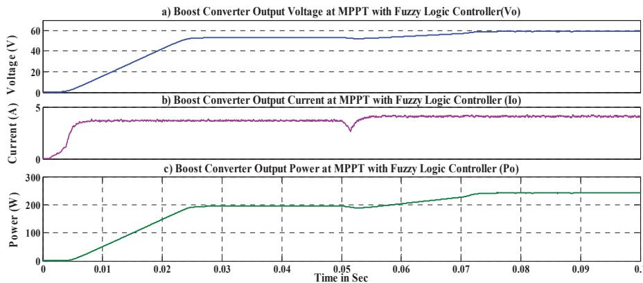
Fig. 10 Boost Converter output at MPPT with FLC
