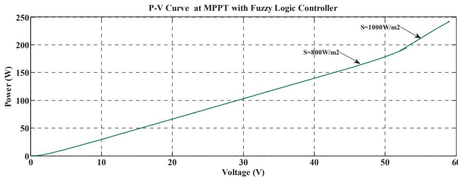
Fig. 11 P-V Characteristics at MPPT with FLC
