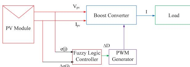
Fig. 3 Block diagram of FLC based MPPT
