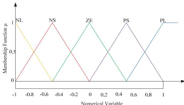
Fig. 6 Membership function for inputs of FLC
