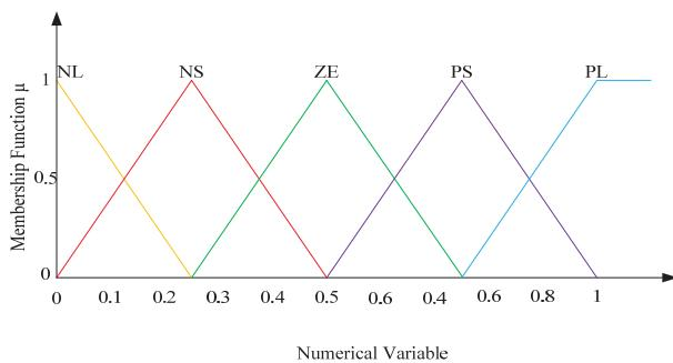
Fig. 7 Membership function for output of FLC
