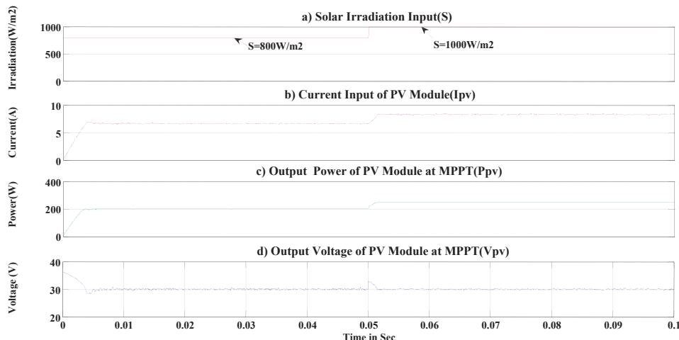
Fig. 8 Response of a PV Module at MPPT
