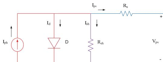
Fig. 1 Equivalent circuit of a PV cell
