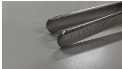
Fig. 8 Vibrating fork A3B1C1
