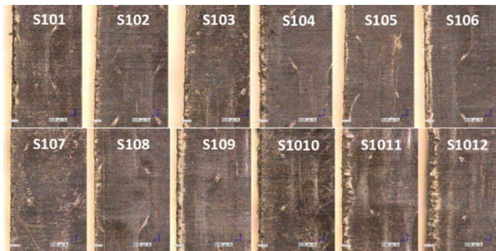
Fig. 13 Increasing damage on the surface ply of short beam samples (strip S10)
