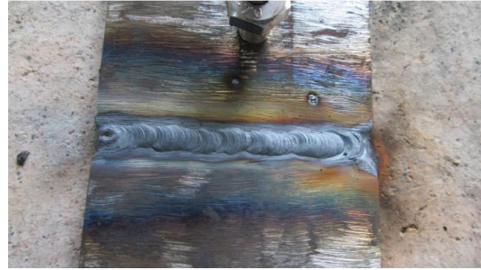
Fig. 5 A close view of weld bead and heat affected zone
