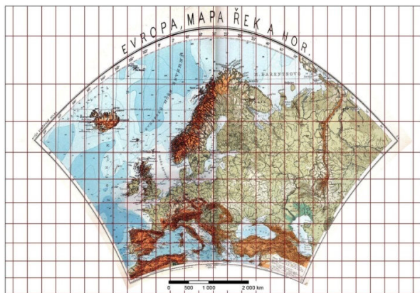
Fig. 15 Properly georeferenced map (into Albers projection) reprojected in Mercator projection
