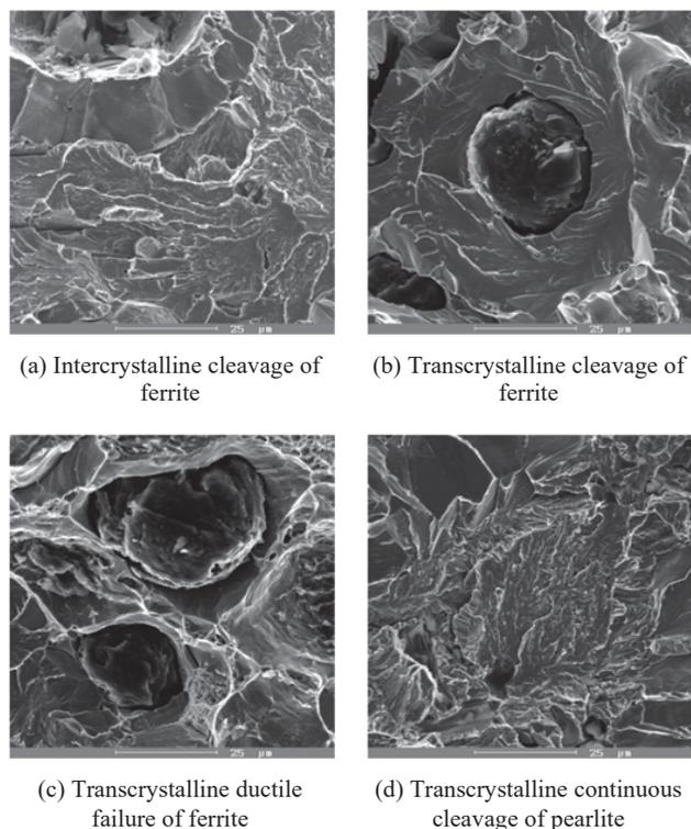
Fig. 7 Failure micromechanisms at impact stress, SEM
