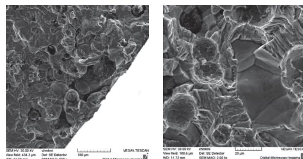
(a) Initiation of fatigue failure
