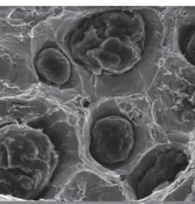
(c) Transcrystalline ductile failure of ferrite
