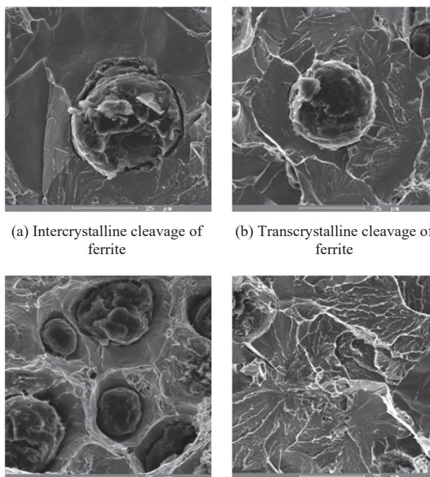
(a) Intercrystalline cleavage of ferrite
