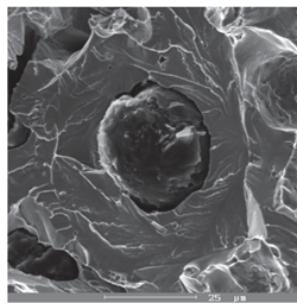
(b) Transcrystalline cleavage of ferrite
