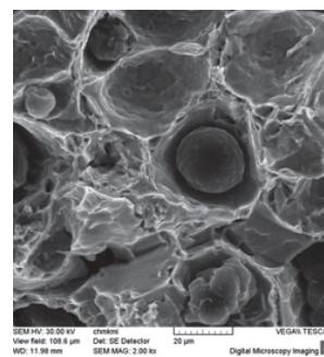
(c) Final rupture – transcrystalline ductile failure
