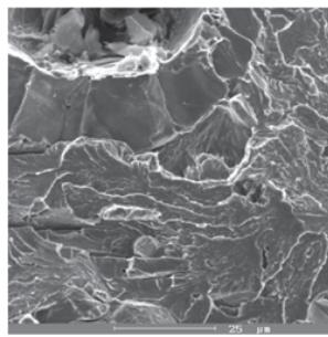
(a) Intercrystalline cleavage of ferrite
