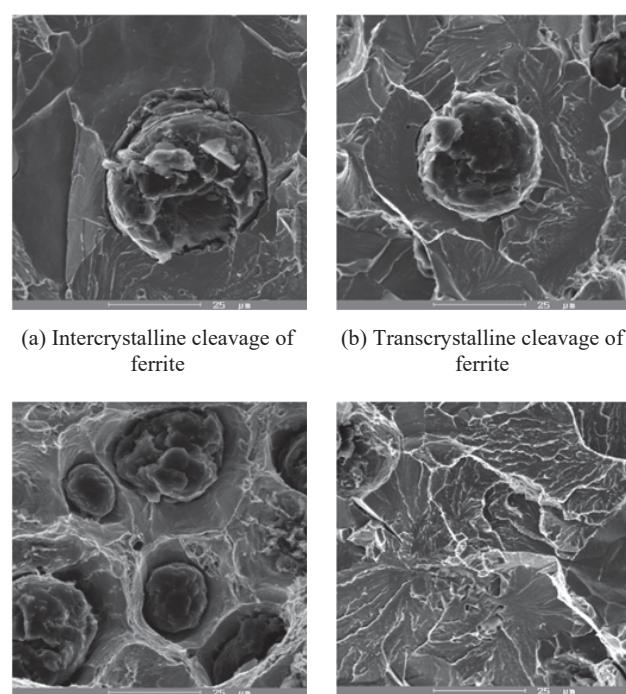
Fig. 6 Failure micro mechanisms at static stress, SEM
