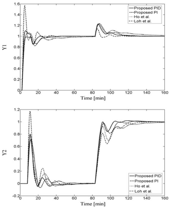
Fig. 3 Closed-loop time responses for WB column.
