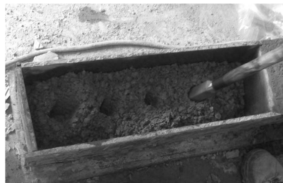
Fig. 4 Attempt to vibrate carbon fibers
