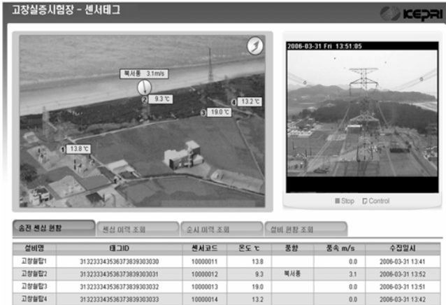
Fig. 5 Web screen of transmission tower monitoring system
