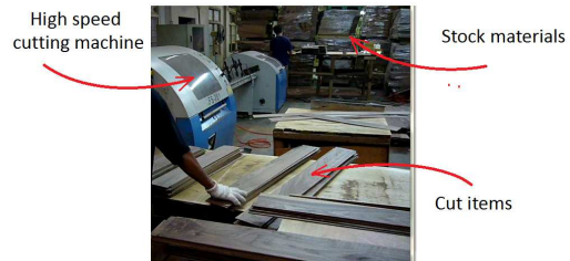
Fig. 1 A production line for high-speed floorboard cutting
