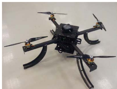
Fig. 1 Designed and Manufactured Quadrotor
