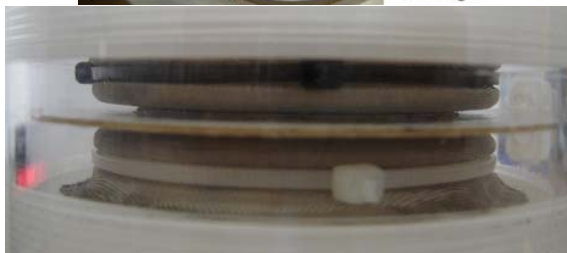
Fig. 5 Cardboard ring with silica gel balls
