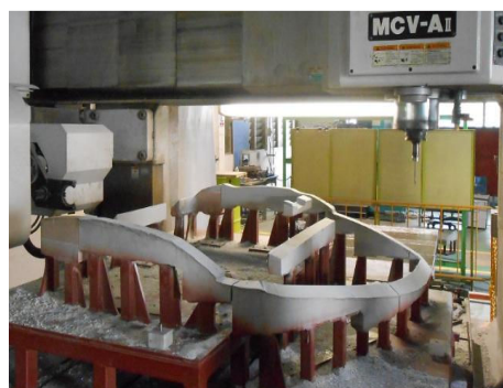
Fig. 1 Milling process for car door checking fixture
