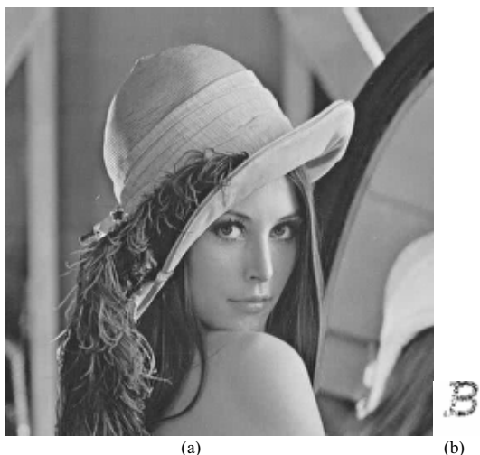
Fig. 5. (a) JPEG Compressed (Quality factor = 10) OPT watermarked image, (b) Extracted watermark from Figure 5(a).
