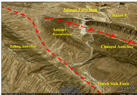
Fig. 2 Satellite image of Salman Farsi dam project constructing on the northern flank of Changal Anticline at the Zagros folded belt
