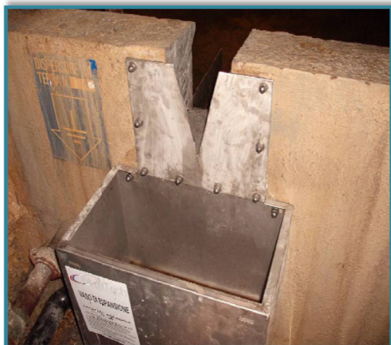
Fig. 3 Weirs used to monitor tunnel inflows
