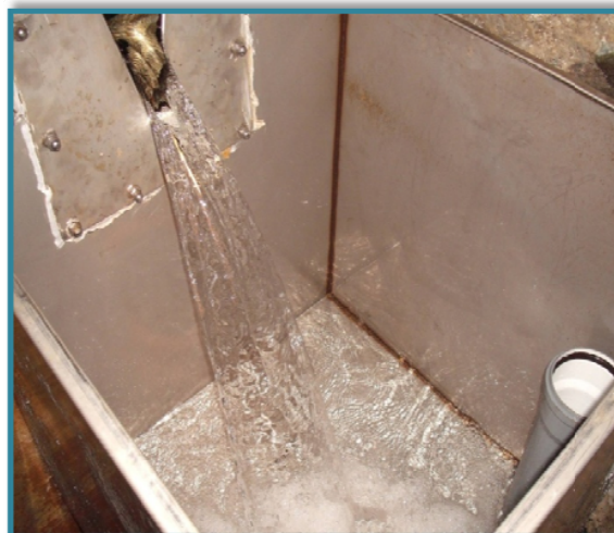
Fig. 3 Weirs used to monitor tunnel inflows
