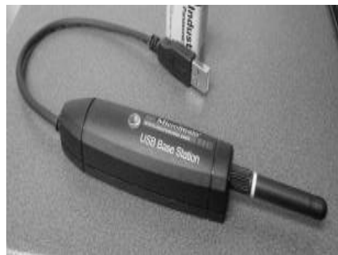
Fig. 3 Wireless Radio Frequency Basestation
