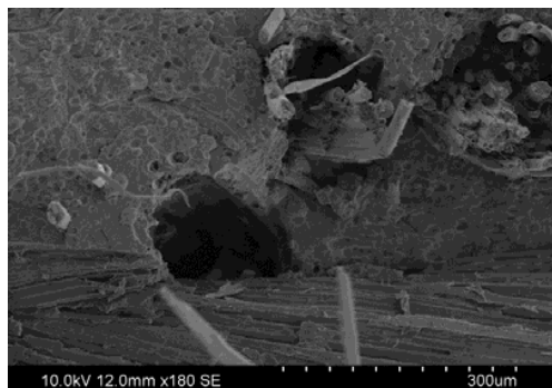
Fig. 4 Tensile fracture surface showing fibre bundle pull-out observed under SEM
