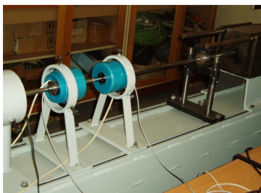
Fig. 2 The Split Hopkinson Pressure Bar
