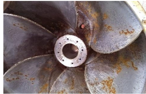
Fig. 16 Cavitation of Impeller
