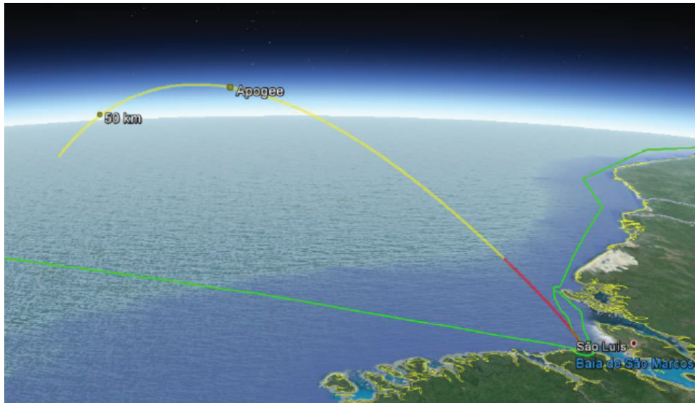
Fig. 2 Planned launch trajectory from CLA: Both the EFTV+ESM are planned to be released together from the rocket stage at an altitude of 90 km
