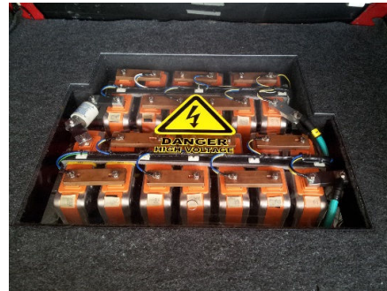
Fig. 4 Battery module arrangement within the EV boot
