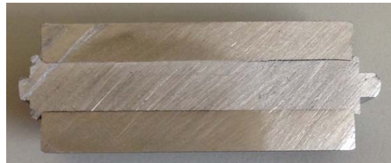
Fig. 8 Cross section shape after forming in forging experiment
