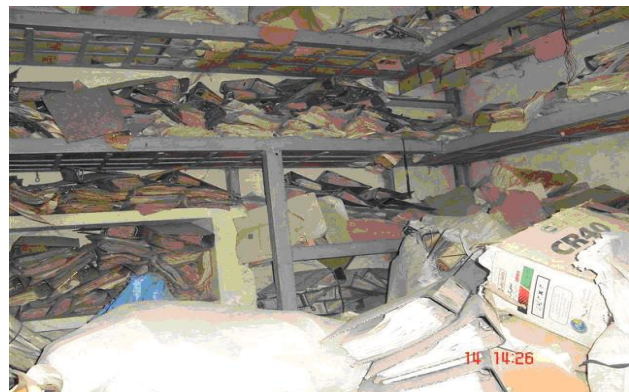
Fig. 9 Unsafe storage of material in racks
