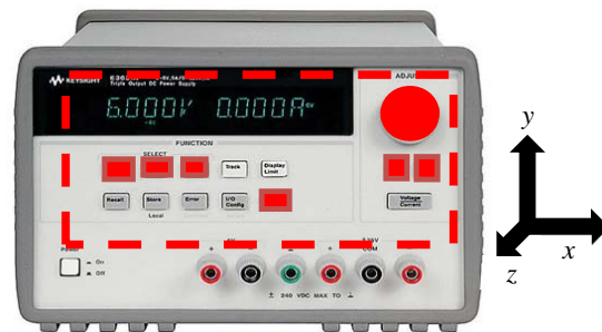
Fig. 8 Power supply control areas
