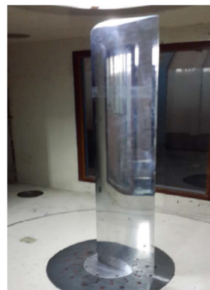
Fig. 3 Half model tested in IIUM-LSWT
